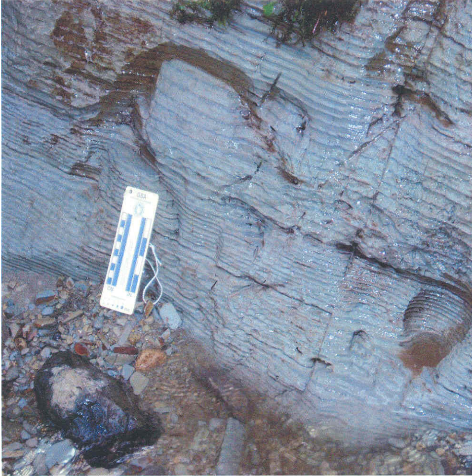
Photo 1: Transitional beds (Qtb) exposed in Tuck Creek. The outcrop of this unit is associated with widespread landsliding in the Tuck Creek ravine.
